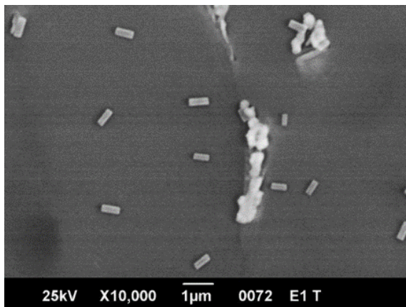
Figure 9. SEM micrograph showing \text{Al}_6\text{-}_7\text{Mn} precipitates in DC samples
