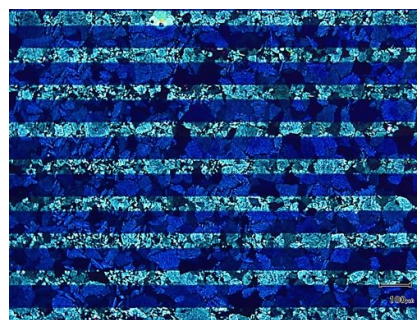
Figure 4. Photograph obtained by optical microscopy of a typical film of the DB-TTF and PS10k composite material in a 1:3 ratio; the angle between the polarizer and the analyzer is 90°
