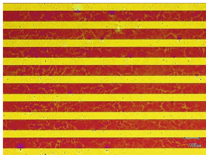
Figure 3. Photograph obtained by optical microscopy of a typical film of the DB-TTF and PS10k composite material in a 1:3 ratio; the angle between the polarizer and the analyzer is 0°
