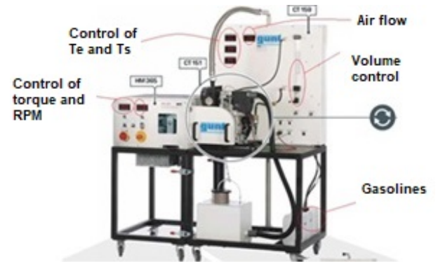
Figure 4. Experimental bench. Air-cooled gasoline engine with 1 cylinder, and HM 365 universal drive and brake unit
