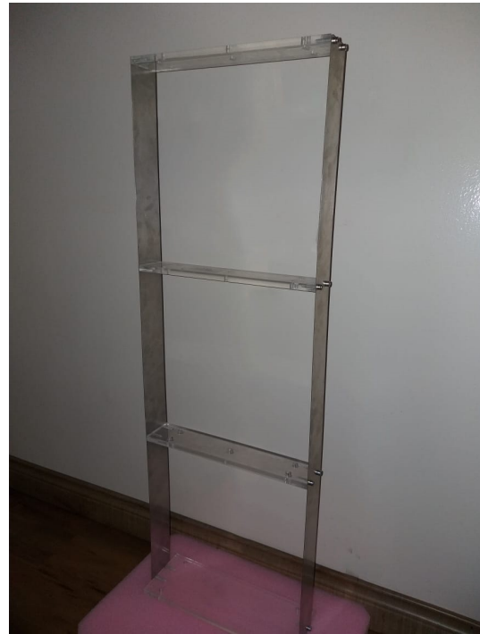
Figure 10. Experimental model of the model with 3 degrees of freedom
